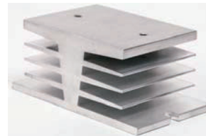
Model: MW-E-52 Size: 52mm*74mm*40mm For 40 amps SSR Mounting method: Panel mount or din rail mount with din rail adaptor
